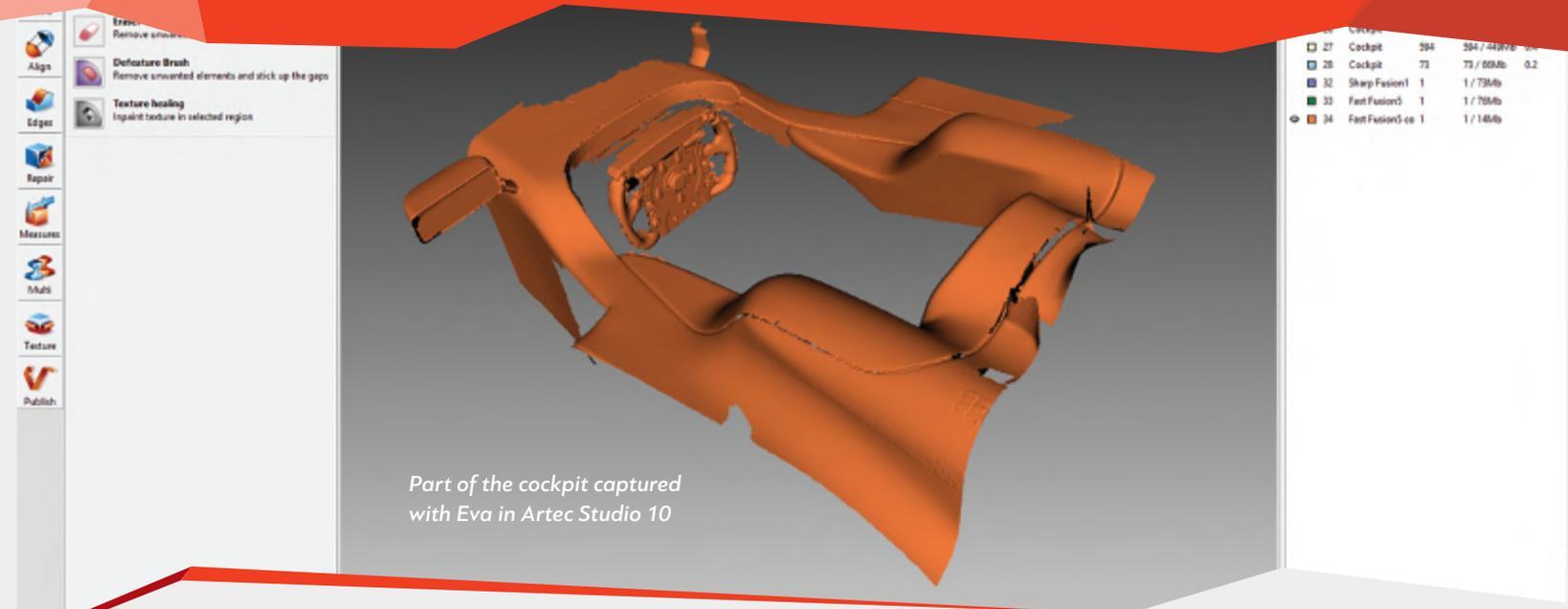
The car was 3D scanned in the owner's reception area and workshop; both areas had good stable lighting but no direct sunlight because this would affect the data capture. There were some dark carbon fibre areas around the wishbones – those were sprayed very lightly. Light reflections around the spoiler areas were also sprayed lightly to ease and quicken the capture. Paul recommends a few tips on how to capture car parts easier.
