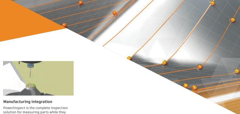
PowerInspect is the complete inspection solution for measuring parts while they are still on the machine, also known as 'On Machine Verification' (OMV). Machine tool probing allows you to make informed scrap or rework decisions quickly.
